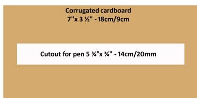
1. Build as many layers of corrugated cardboard cut to the size **7"x 3 1/2" - 18cm/9cm**, up to (**9/16<sup>th</sup> - 14mm**) in thickness. This is the approx' thickness of the pen.
